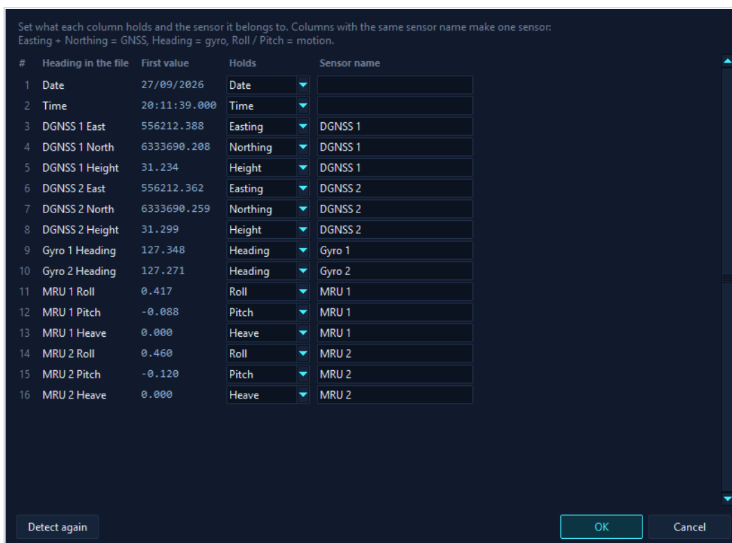
The Columns window: what each column holds and the sensor it belongs to.
