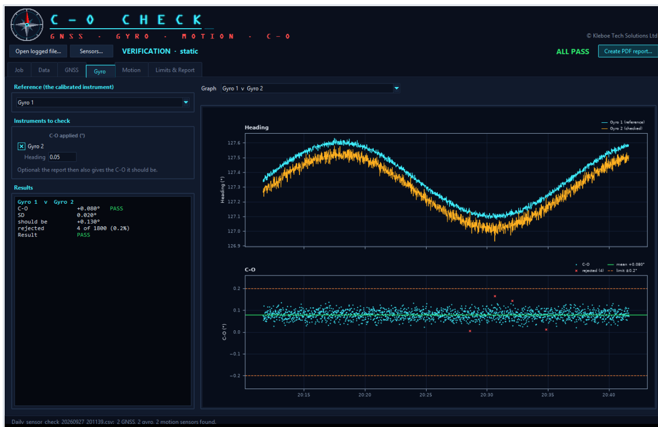
The Gyro tab in a verification, with the C-O applied to Gyro 2 entered.
