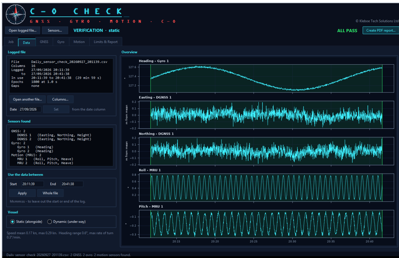
The Data tab: the file, the sensors found, the time window and an overview of the log.
