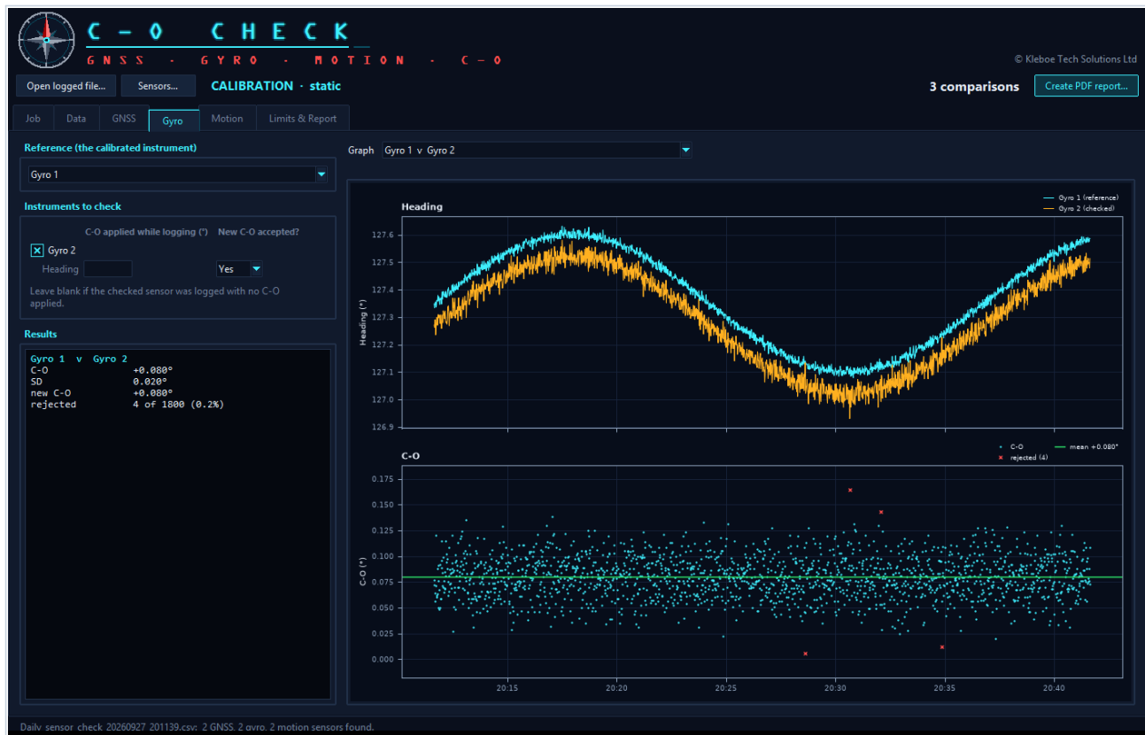
The Gyro tab in a calibration: the new C-O, and New C-O accepted? for the report.
